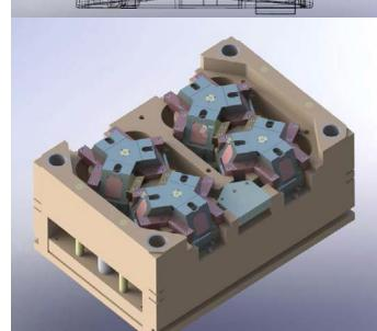
Complex Molds and Tooling are designed with 3-D CAD Software.
