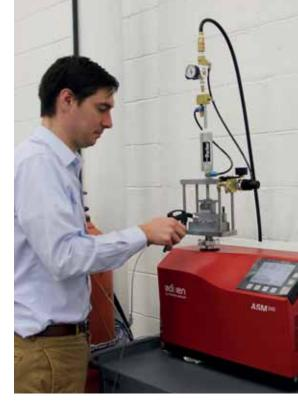
SUPERB engineer performs a helium leak test on an engineered component with a 1x10<sup>-7</sup> mbar liters/second leak specification.
