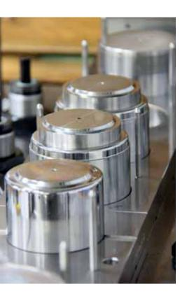
Skilled grinders can hold tolerance to twenty millionth of an inch using grinding machines in a climate controlled environment.
