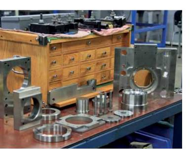
Die components are engineered for full interchangeability and manufactured to exacting tolerances.
